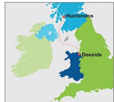
Fig. 8 – 2200 MW subsea HVDC-link bypassing the bottleneck
